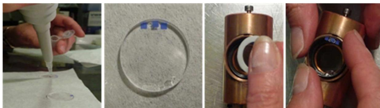
Figure 4 Assembly of demountable 0.01 cm quartz cell of type QS124 (Hellma GmBH, Germany).
