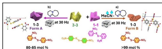
Figure 14 Effect of milling conditions on the 1-1 + 3-3 disulfide exchange in the presence of DBU. Under NG conditions (left), the reaction yields mostly Form A of 1-3 (80–85 mol%), with 15–20 mol% unreacted 1-1 and 3-3. Under LAG conditions (right), Form B of 1-3 is obtained quantitatively. 41, 53
