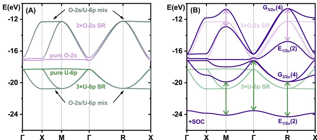
Fig. 5 Band structure of  $\delta$ -[UO<sub>3</sub>] in the U-6p/O-2s semi-core region. Energies in eV, lower Fermi edge set to zero. PBE calculations with VASP. (Left) (A) Projected SR bands, U-6p in green, O-2s in lilac. (Right) (B) SO split bands in purple, and transparent spin-averaged SR bands: dominantly U-6p in green and dominantly O-2s in lilac. Green and lilac double-arrows highlight the SO splitting.
