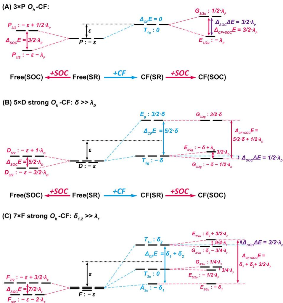
Fig. 4  $O_h$ -Crystal-field and spin-orbit effects on p, d and f orbital levels. (Top) (A) p-Shell – independent shift  $\varepsilon$  by the CF and splitting  $3/2 \cdot \lambda_p$  by SOC. (Middle) (B) d-Shell – shift  $\varepsilon$  and splitting  $5/2 \cdot \delta$  by the CF, partially quenching the  $5/2 \cdot \lambda_D$  SO splitting. (Bottom) (C) f-Shell – shift  $\varepsilon$  and splitting  $\delta_1, \delta_2$  by CF, significantly quenching the  $7/2 \cdot \lambda_f$  SO splitting.
