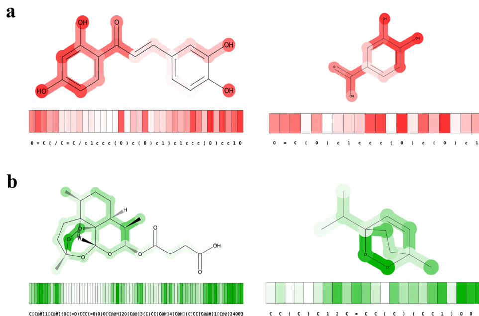
Fig. 2 Attention heat map of molecules with (a) antioxidant activity and (b) molecules with oxidant activity. BERT's attention scores are allocated to both SMILES tokens and structural representation. Darker colors indicate higher attention scores.
