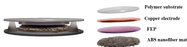
Figure 2. Schematic representation of ABS-based TENG
