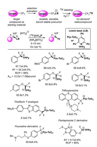
Fig. 14 Synthesis of fluorine-18 labelled  $CF_3$  and  $CF_2H$  groups is possible via FLP selective activation followed by Lewis base substitution with  $[^{18}F]F^-$ . This methodology greatly simplifies the radiosynthesis of the fluorine-18 isotopologues as it allows the non-labelled target compound to be used as a starting material. Yields correspond to radiochemical conversions (RCC). See ref. 44 for details.
