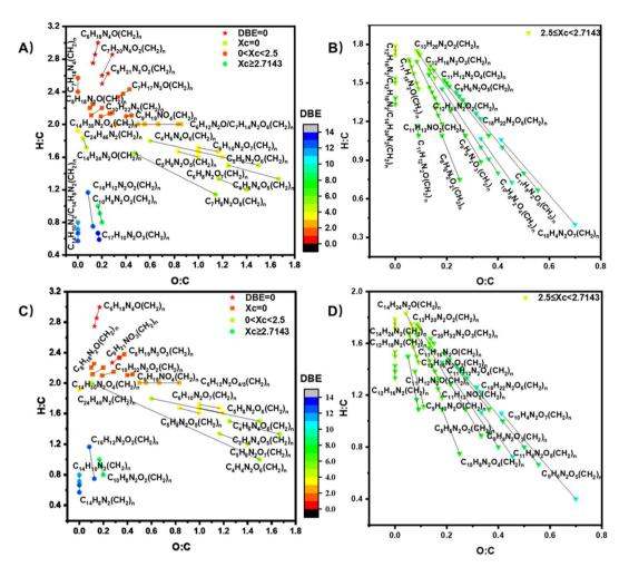
Fig. 3 Van Krevelen plot for homologous series of CHON compounds produced from the ozone oxidation reaction (A and B) and photooxidation reaction (C and D). The "n" refers to the number of CH<sub>2</sub> groups in a given family.
