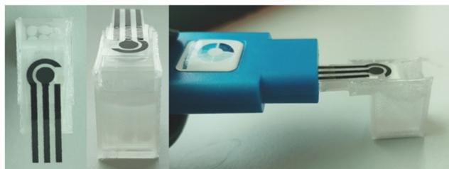
**Fig. 6** Three-dimensional printed case for the integration of the printed electrode and alginate spheres.
