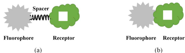
Fig. 3 Fluorescent sensor model (a) with and (b) without a spacer.
