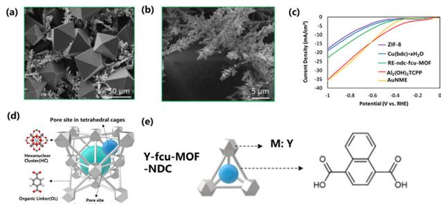
**Fig. 9** SEM images of RE-ndc-fcu-MOF on AuNME before (a) and after electrochemical reaction (b). (c) Linear sweep voltammetry (LSV) scans (0 to  $-1$  V vs. RHE,  $0.1$  M  $\text{KHCO}_3$ ) of different MOF@AuNMEs and AuNME control, Copyright 2018, American Chemical Society. (d) Microscopic diagram of fcu-MOF-BDC. (e) The metal node of MOF is replaced with Y to get Y-fcu-MOF-BDC, Copyright 2020, American Chemical Society.
