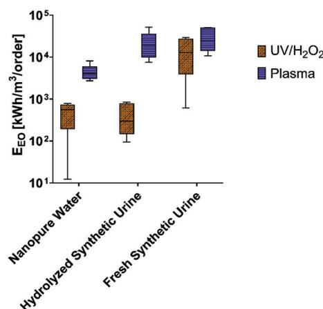
Fig. 4 Calculated electric energy per order ( $E_{EO}$ ) (kW h m<sup>-3</sup> per order) for both bench-scale reactors in the nanopure water and synthetic urine matrices. The box and whisker plot displays 95% confidence intervals for  $E_{EO}$  values ( $n = 6$ , all pharmaceutical compounds in each data point).
