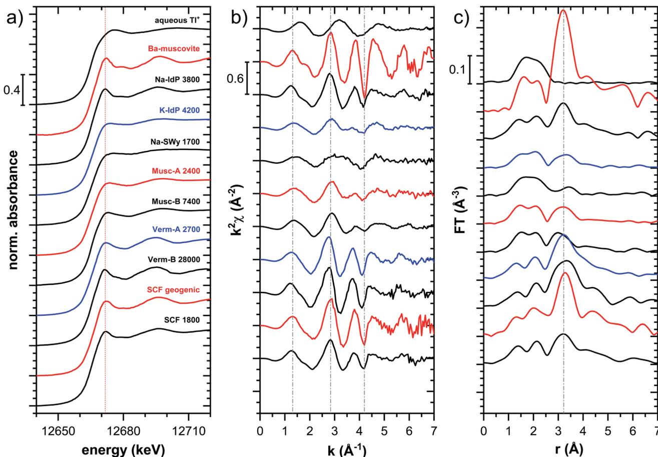
Fig. 4 Tl  $L_{III}$ -edge XANES (a), EXAFS (b) and Fourier-transformed EXAFS (c) spectra of selected Tl-loaded illite (Na-IdP; K-IdP), smectite (Na-SWy), muscovite (Musc-A; Musc-B), and vermiculite (Verm-A; Verm-B) samples and of a soil clay fraction (SCF) with geogenic Tl and with additional sorbed Tl. Numbers in spectra labels indicate the Tl loading of the respective phyllosilicate in mg kg<sup>-1</sup>. Vertical lines serve to guide the eye.
