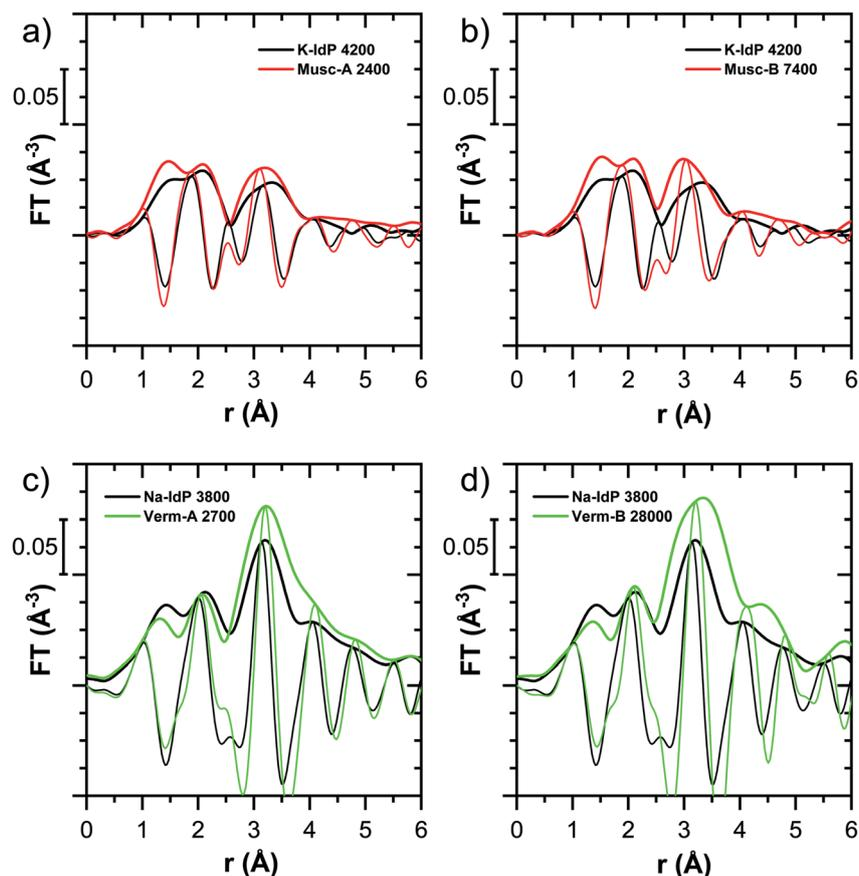
Fig. 7 Fourier-transformed  $k^2$ -weighted Tl  $L_{III}$ -edge EXAFS spectra of (a and b) Tl-loaded muscovites Musc-A and Musc-B compared to Tl-loaded K-IdP and of (c and d) Tl-loaded vermiculites Verm-A and Verm-B compared to Tl-loaded Na-IdP. Numbers in sample names indicate the Tl loading of the phyllosilicates in  $\text{mg kg}^{-1}$ .
