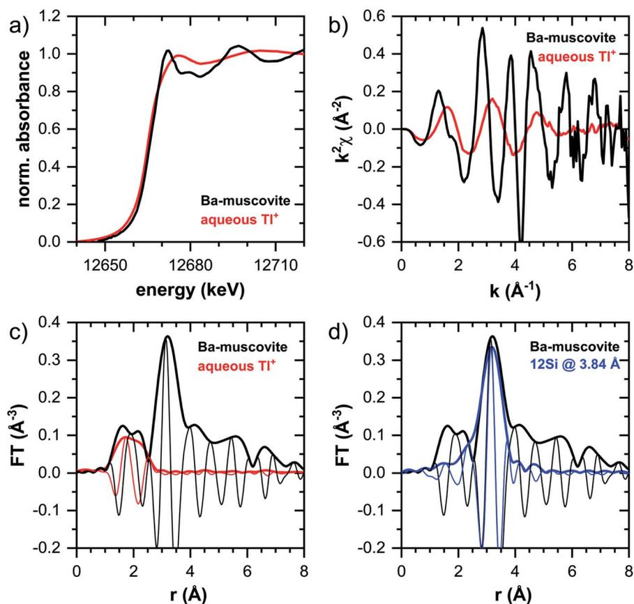
Fig. 3 XANES and EXAFS reference spectra of Tl-rich Ba-muscovite and of 10 mM aqueous  $Tl^+$ : (a) XANES spectra, (b)  $k^2$ -weighted EXAFS spectra, (c) Fourier-transform of  $k^2$ -weighted EXAFS spectra (magnitudes: thick lines; imaginary parts: thin lines). (d) Fourier-transform of EXAFS spectrum of Tl-rich Ba-muscovite compared with shell-fit involving 12 Si atoms at a distance of 3.84 Å from Tl.
