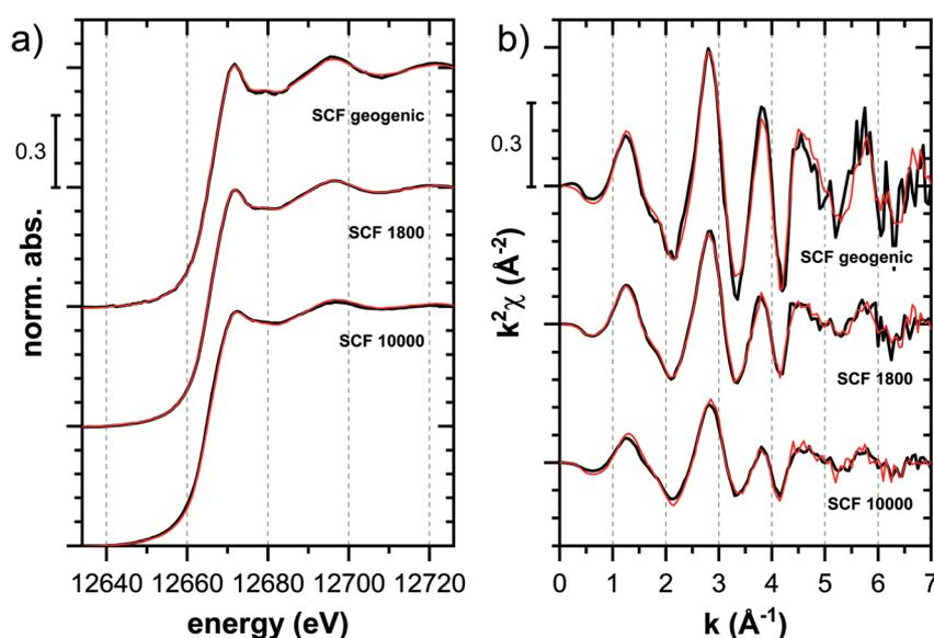
Fig. 8 Tl  $L_{\text{III}}$ -edge (a) XANES and (b) EXAFS spectra of a soil clay fraction (SCF) with  $\sim 260 \text{ mg kg}^{-1}$  geogenic Tl (SCF geogenic) and with an additional 1800  $\text{mg kg}^{-1}$  (SCF 1800) or 10 000  $\text{mg kg}^{-1}$  freshly adsorbed Tl (SCF 10000) (black lines) and linear fit reconstructions (red lines). LCF results are listed in Table 2.
