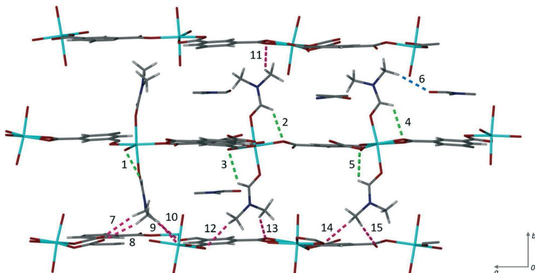
Fig. 3 Hydrogen bonding in **1**. The three types found within the structure are shown in different colours: blue shows the hydrogen bond (6) between the coordinated DMF and the solvent DMF, green the intramolecular hydrogen bonds (1–5) from the coordinated DMF to the carboxylate oxygen, and pink the hydrogen bonds (7–15) between the axially bound DMF molecules to the carboxylate oxygen atoms of subsequent layers. The numbers correspond to those given in Table S2.†
