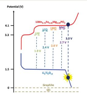
Scheme 1 Potential of the electrode materials used for constructing a full cell.
