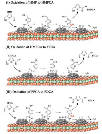
Fig. 7 View of the plausible reaction mechanism of oxidation of 5-HMF to FDCA over Pd/HT catalysts. Reprinted with permission from ref. 122, Copyright @ 2016 American Chemical Society.
