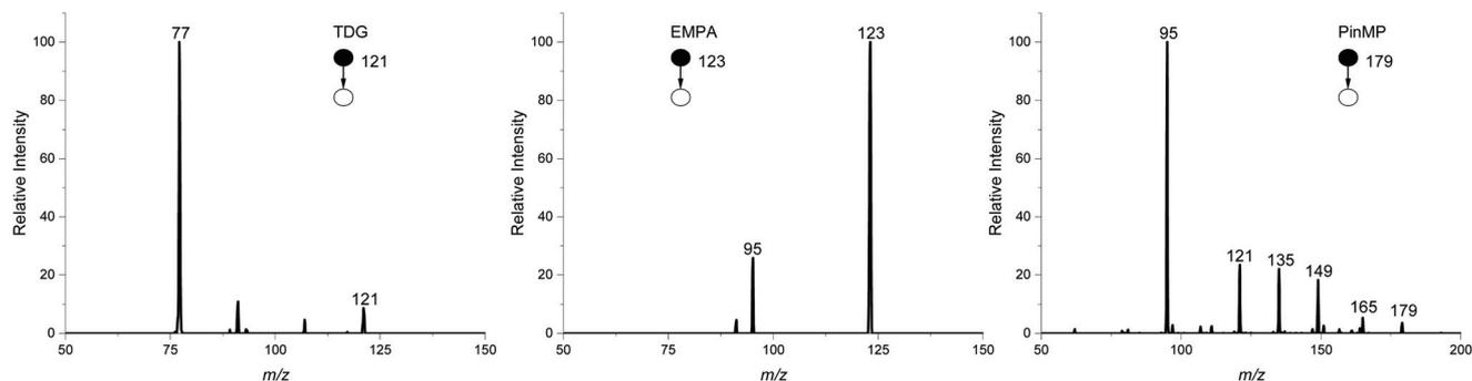
**Fig. 2** MS/MS spectra for CWA hydrolysis products at their respective empirical LODs on the benchtop ion trap instrument. The  $[M - H]^-$  peak was isolated and fragmented in  $MS^2$  for all CWA hydrolysis products.
