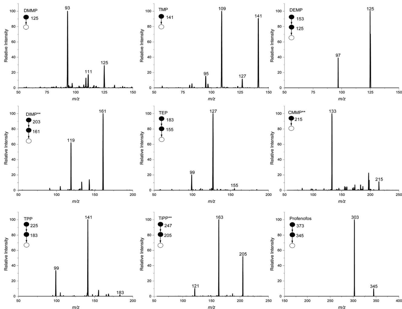
**Fig. 1** MS<sup>n</sup> spectra of CWA simulants at their respective empirical LODs on the benchtop ion trap instrument. The [M + H]<sup>+</sup> peak was isolated for all CWA simulants except DIMP, CMMP, and TiPP which the sodium adduct [M + Na]<sup>+</sup> was isolated and fragmented. The use of the sodium adduct is indicated by \*\* next to the compound name.
