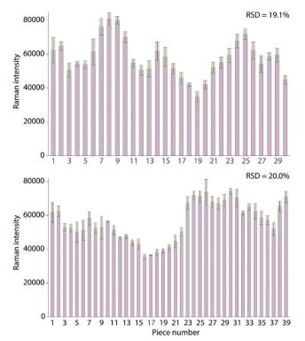
Fig. 5 SERS intensity of the 268 cm<sup>-1</sup> band in each of the pieces cut from prepared films A (top) and B (bottom). Each data point represents the average value from five SERS spectra and error bars show the RSD. The RSD of the average values were 19.1% for film A and 20.0% for film В
