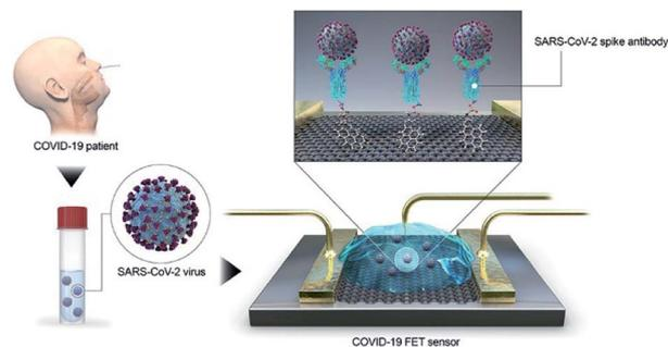
Fig. 4 Schematic diagram of COVID-19 FET sensor operation procedure.<sup>40</sup>
