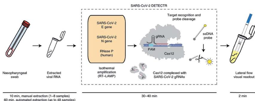
Fig. 3 Schematic of CRISPR-Cas12-based assay workflow for detection of SARS-CoV-2.<sup>19</sup>
