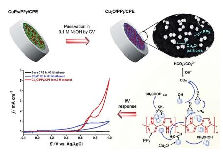
Fig. 14 The preparation of  $Cu_2O/PPy/CPE$  for ethanol electrocatalytic oxidation. Reproduced with permission from ref. 128. Copyright 2020 Elsevier.
