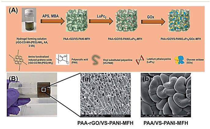
Fig. 9 (A) The PAA-rGO/VS-PANI/LuPc2/ $GO_x$ -MFH synthesis procedure. (B) SEM images of (a) PAA-rGO/VS-PANI-MFH, and (b) PAA/VS-PANI-MFH. Reproduced with permission from ref. 90. Copyright 2017 Elsevier.
