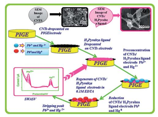
Fig. 7 Fabrication procedure for the electrochemical sensor for the simultaneous determination of Hg(II) and Pb(III). Reproduced with permission from ref. 78. Copyright 2018 Elsevier.
