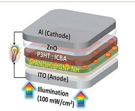
Fig. 11 BHJ PSC with the tool architecture: ITO/SPAN(SH)@GNP(X%) NH/P3HT; ICBA/ZnO/Al. Reproduced with permission from ref. 107. Copyright 2018 Elsevier.
