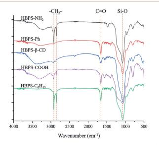
Fig. 1 FT-IR spectral characterization of HBPS-NH $_2$ , HBPS-Ph, HBPS- $\beta$ -CD, HBPS-C $_6$ H $_1$ 3 and HBPS-COOH.
