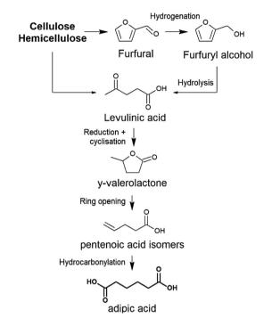
Fig. 17 Catalytic route for the production of adipic acid from hemicellulosic and cellulosic sugars via GVL proposed by Han et al. <sup>439</sup>
