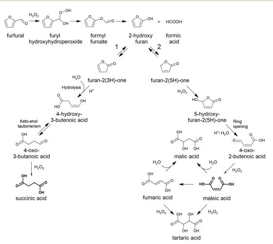
Fig. 14 Oxidation of furfural with H<sub>2</sub>O<sub>2</sub> in the liquid phase using Brønsted acid or basic catalysts.
