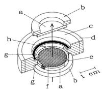
**Fig. 2** Schematic representation of the IR-SEC cell. The arrow represents the propagation of the IR-light beam (a) IR-transparent  $CaF_2$  window mounted onto a (b) Plexiglas ring, (c) Teflon body, (d) steel surround, (e) Pt counter electrode, (f) the mesh working electrode, (g) O-ring, (h) capillary connection to the reference electrode. Reprinted from the original work by Moss *et al.*, <sup>11</sup> Copyright 1990, with permission from John Wiley and Sons.
