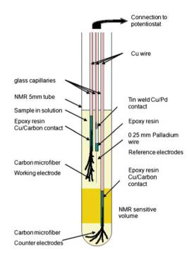
**Fig. 15** Schematic of a three-electrode NMR-SEC cell with carbon microfibre WE and CE placed above and below the NMR detection area. Reprinted by permission from Springer Nature: from the original work by Bussy *et al.*, <sup>261</sup> Copyright 2012.
