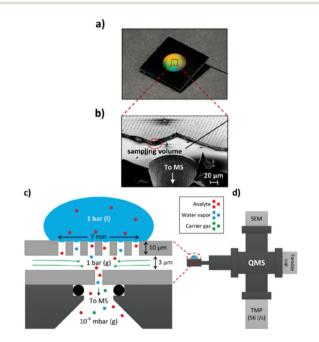
Fig. 24 Membrane DEMS setup for thin-layer cell; (a) membrane chip photograph; (b) scanning electron microscope image of the membrane chip; (c) schematic of the membrane chip; (d) schematic of the setup. Image reprinted and modified with permission from Trimarco et al. 301 Copyright 2018 American Chemical Society.
