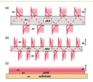
**Fig. 8** Schematic representation of the evanescent wave/field with an ever decreasing IRE thickness. As one can see in (a) and (b), the smaller IRE has more reflections than the bigger IRE. When the size is small enough, as one can see in (c), a waveguide is created with a continuous evanescent field. Reprinted from the original work by Schadle and Mizaikoff, <sup>68</sup> Copyright 2016, with permission from SAGE Publications.
