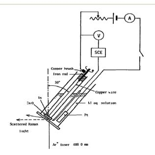
**Fig. 12** Rotating Raman-SEC device. Reprinted from the original work by Yamada *et al.*, <sup>154</sup> Copyright 1978, with permission from Elsevier.
