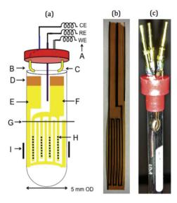
**Fig. 16** Schematic and photograph of an NMR-SEC cell with interdigitated WE and CE placed in the NMR detection area. Reprinted from the original work by Sorte *et al.*, <sup>269</sup> Copyright 2016, with permission from Elsevier.
