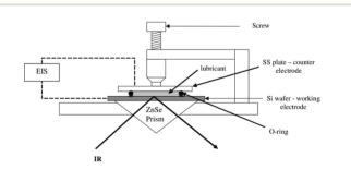
**Fig. 5** Schematic of an optically transparent electrode ATR IR-SEC setup, in a single bounce configuration. Reprinted with permission from Springer Nature: from the original work by Purushothaman *et al.*,<sup>70</sup> Copyright 2012.
