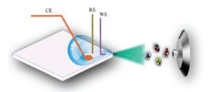
Fig. 21 D Schematic of the droplet-based EC-MS approach. Reprinted with permission from Yu  $et\ al.^{292}$  Copyright 2018 American Chemical Society.
