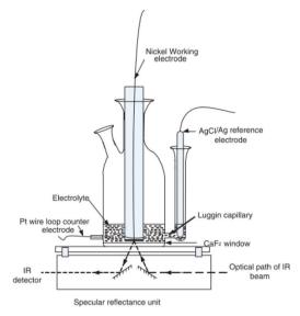
**Fig. 3** Schematic representation of a reflection setup. Republished with permission of Journal of The Electrochemical Society, original by Alwis *et al.*, <sup>14</sup> Copyright 2013; permission conveyed through Copyright Clearance Center, Inc.
