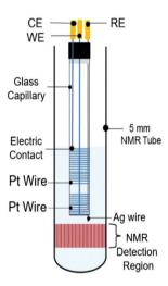
Fig. 18 Schematic of a coil-based three-electrode NMR-SEC cell. Reprinted from the original work by da Silva *et al.*,<sup>275</sup> Copyright 2019, with permission from Elsevier.
