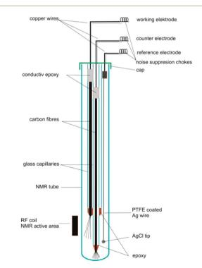
Fig. 14 Schematic of a three-electrode NMR-SEC cell with carbon fibre WE and CE, partially placed in the NMR detection area. Reprinted with permission from Klod et al.<sup>253</sup> Copyright 2009 American Chemical
