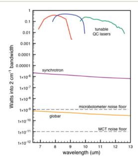
Fig. 7 Comparison of Weida and Yee of three different IR sources of the signal through a 10  $\mu m$  pinhole. 96 Reprinted and adapted from the original work by Weida and Yee, 96 Copyright 2011, with permission from SPIE and M. Weida.
