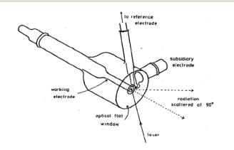
**Fig. 10** Example of a stationary electrochemical cell used for Raman experiments. Reprinted from the original work by Fleischmann *et al.*, <sup>120</sup> Copyright 1974, with permission from Elsevier.
