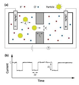
Fig. 3 (a) Schematic representation of a resistive pulse sensing system. (b) The current transient properties upon particles passing through the
