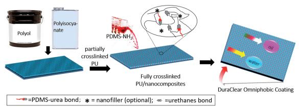
Scheme 2 Schematic illustration of the omniphobic PU coatings preparation using our novel top-layer approach.
