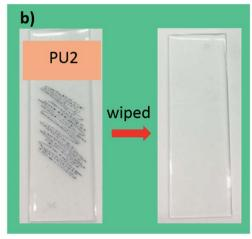
Fig. 6 Ink traces left behind by a permanent ink marker on PU1- and PU2-coated glass plates. Photos were taken before and after the samples had been subjected to wiping treatment are also shown.
