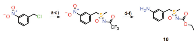
Scheme 6 Synthesis of key sulfoximine building block 10 in the initial preparation of atueveciclib. Reagents and conditions: (a) NaSMe, EtOH, -15^{\circ}\text{C} to rt, crude; (b) \text{H}_5\text{IO}_6 , \text{FeCl}_3 , MeCN, rt, 70%; (c) \text{CF}_3\text{C(O)NH}_2 , PhI(OAc) 2 , MgO, [\text{Rh}_2(\text{OAc})_4] , DCM, rt, 99%; (d) \text{K}_2\text{CO}_3 , MeOH, rt, 79%; (e) \text{ClC(O)OEt} , pyridine, 0^{\circ}\text{C} to rt, crude; (f) \text{TiCl}_3 , THF, rt, crude.
