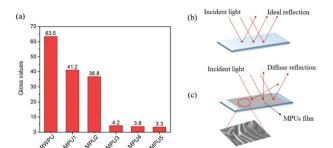
Fig. 6 Gloss values and matting mechanism. (a) The gloss values of the MPU-based films, (b) mirror-like surface with high gloss, and (c) rough surface with matting effect.
