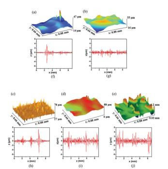
Fig. 8 3D profilometer images and line scanning curves of the MPU films. Surface area roughness of (a) MPU1, (b) MPU2, and (c) MPU3, (d) MPU4, and (e) MPU5 with  $R_{\alpha}$  values of (a) 0.25, (b) 0.56, (c) 0.97, (d) 1.3, and (e) 2.3 μm, respectively. Line roughnesses of (f) MPU1, (g) MPU2, (h) MPU3, (i) MPU4, and (j) MPU5, where the  $\lambda_a$  values are (f) 7.0, (g) 7.4, (h) 7.8, (i) 10.2, and (j) 12.9 µm, respectively.
