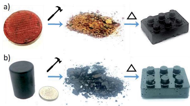
Fig. 6 Sulfur polymer samples on, after breaking into powder, centre, and then after being reformed into a monolith again, right: (a) sulfur–perillyl alcohol copolymer, and (b) sulfur–squalene copolymer. Both samples were made with 50 wt% sulfur.
