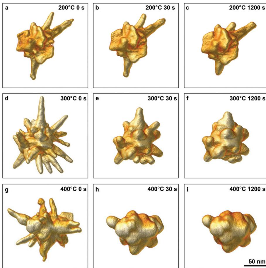
**Fig. 3** 3D visualizations, using fast tomography, of an Au NS before (a) and after heating for 30 s (b) and 1200 s (c) at 200 °C. 3D visualizations for the same time steps are shown for 300 °C (d–f) and 400 °C (g–i).
