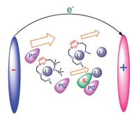
Scheme 5 The electrochemical behaviors of  $\bf 5$  and  $\bf 6$  as electrolytes for LIBs.  $^{28}$
