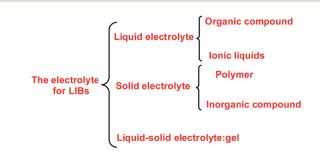
Scheme 1 The electrolytes for lithium ion batteries.
