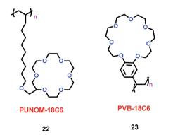
Scheme 12 The structures of crown ethers-based polymers. 35
