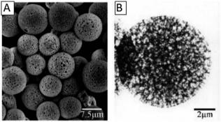
Fig. 4 SEM (A) and TEM (B) images of the hollow core/porous shell of PVAc. Reproduced from ref. 73 with permission from John Wiley and
