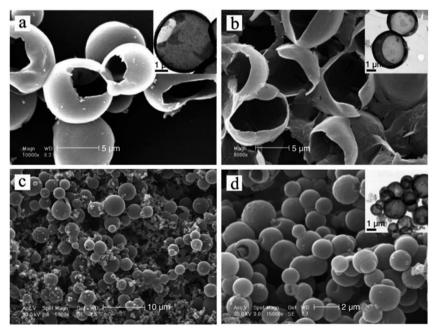
Fig. 7 SEM images of poly(o-toluidine) (POT) hollow microspheres synthesized at different [APS]/[o-toluidine] ratios of: (a) 0.8:1 and (b) 0.6:1. (c) and (d) SEM images of POT hollow microspheres synthesized at different temperatures: (c) 25 °C and (d) -10 °C. The insets show the corresponding TEMs image of the POT hollow structures. Reproduced from ref. 76 with permission from John Wiley and Sons.
