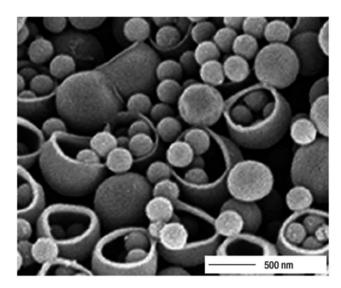
Fig. 6 Demonstration of the possibility to load bowl-shaped PS particles with solid PS beads of 260 nm diameter. Reproduced from ref. 75 with permission from the Nature Publishing Group.
