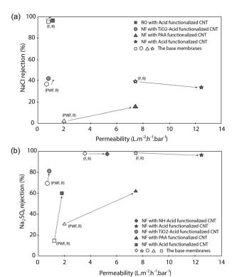
Fig. 9 Permeability vs. rejection of a functionalized CNT membrane. (a) NaCl rejection and (b)  $Na_2SO_4$  rejection (data from ref. 69, 73, 76, 83, 87 and 88; F: permeability of salt solution; PWF: permeability of pure water; R: salt rejection).
