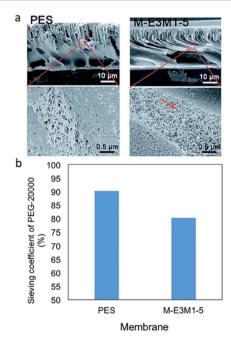
Fig. 6 Cross-section SEM images of PES and M-E3M1-5 (PES with CNT-polymethyltriethyl ammonium chloride and CNT-polyethylene glycol methyl ether methacrylate) (a) and their PEG-20 000 sieving coefficient (b).<sup>78</sup> SEM images are reproduced from ref. 78 with permission from The Royal Society of Chemistry.
