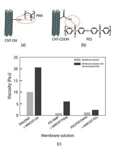
Fig. 4 Hydrogen bonding of functionalized CNT/polymer matrix and its effect on membrane solution viscosity. (a) CNT–OH/PAN, (b) CNT–COOH/PES, (c) solution viscosity of membrane solution and membrane solution containing functionalized CNT (PAN(14%)/DMF/CNT(2%); PSf(18%)/NMP/CNT(2%); PES(21)/PVP/DMAc/CNT(1%)); data from ref. 56, 69 and 90.
