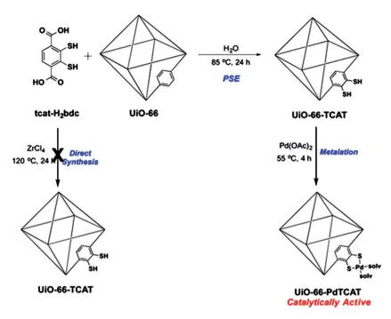
Scheme 20 Schematic view of the synthesis of UiO-66-TCAT and UiO-66-PdTCAT. [Reprinted with permission from ref. 277. Copyright 2015, American Chemical Society.]
