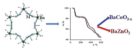
Fig. 36 Preparation of crystalline  $BaCoO_{3-x}$  and  $BaZnO_2$  as a result of solid state thermolysis of the CPs. [Reprinted with permission from ref. 359. Copyright 2015, Elsevier.]
