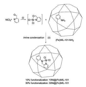
Scheme 19 One-pot synthesis of the MOF-anchored nickel complex Ni@(Fe)MIL-101. [Reprinted with permission from ref. 35. Copyright 2013, American Chemical Society.]
