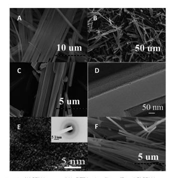
Fig. 30 (A) SEM images of Al–DTPA microfibers; (B and C) SEM images of NCF-900; (D and E) TEM images of NCF-900. Inset is the corresponding selected area electron diffraction pattern of NCF-900; (F) SEM images of  $\gamma\text{-Al}_2\text{O}_3$  obtained by heating Al–DTPA at 800 °C in air. [Reproduced from ref. 305 with permission from The Royal Society of Chemistry.]
