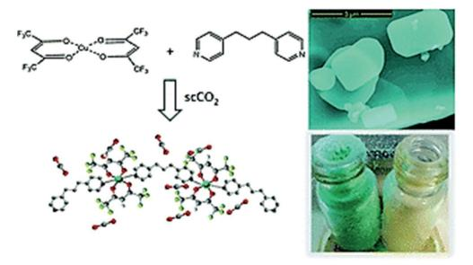
Fig. 21 The preparation of Cu(n) 1D MOFs using an eco-efficient method based exclusively on supercritical  $CO_2$  as a solvent. [Reproduced from ref. 234 with permission from The Royal Society of Chemistry.]
