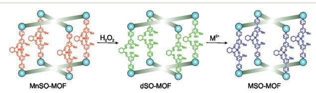
Scheme 23 Demetalation of Mn(III)SO-MOF and its subsequent remetalation. [Reprinted with permission from ref. 285. Copyright 2011, American Chemical Society.]
