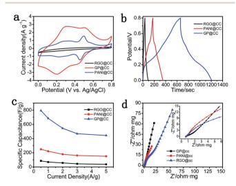
Electrochemical characterization of rGO@cc, PANI@cc and GP@cc electrodes in a 1 M H<sub>2</sub>SO<sub>4</sub> electrolyte, three-electrode system. (a) CV curves at a scan rate of 5 mV s<sup>-1</sup>. (b) Galvanostatic charge/ discharge curves at a current density of 1 A g<sup>-1</sup>. (c) Specific capacitances versus current densities. (d) Nyquist plots with inset showing close-up views of the high-frequency regime.
