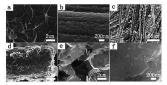
Fig. 1 SEM image of RGO@cc (a), PANI@cc (b) and SEM images of GP@cc (c-f).
