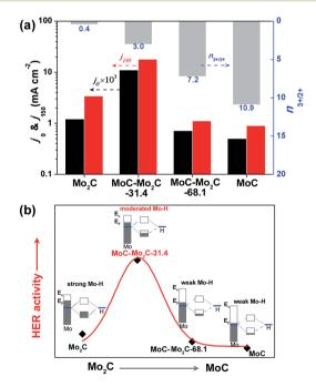
Fig. 4 (a)  $j_0$  (obtained by extrapolating the Tafel curves to  $\eta=0$  mV) and  $j_{150}$  (current density at  $\eta=150$  mV) of the above MoC<sub>x</sub>, which are associated with the ratio of surface Mo<sup>3+</sup>/Mo<sup>2+</sup> determined through XPS analysis. (b) Schematic illustration of the HER activity relying on the electron density of Mo in a series of MoC<sub>x</sub> electrocatalysts.
