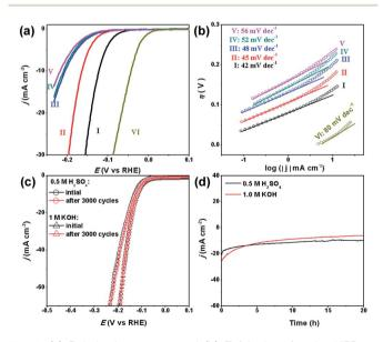
Fig. 5 (a) Polarization curves and (b) Tafel plots for the HER on modified GCEs comprising (l) MoC–Mo<sub>2</sub>C-31.4, (II) Mo<sub>2</sub>C, (III) MoC–Mo<sub>2</sub>C-68.1, (IV) MoC–Mo<sub>2</sub>C-30 (mixed), (V) MoC, and (VI) commercial Pt/C in 1.0 M KOH. (c) Stability of the MoC/Mo<sub>2</sub>C-31.4 modified electrodes with an initial polarization curve and after 3000 cycles in 0.5 M H<sub>2</sub>SO<sub>4</sub> and 1.0 M KOH, and (d) the long-term durability tests at  $\eta=190$  mV.
