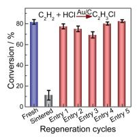
Fig. 7 Relative catalytic activity of acetylene hydrochlorination over the fresh, sintered and regenerated Au/C catalysts. Entries 1–3: sintered Au/C regenerated directly with CHI $_3$  at 40 °C; Entries 4 and 5: sintered Au/C catalyst regenerated with CHI $_3$  containing HAuCl $_4$  (0.002 M) at 40 °C.
