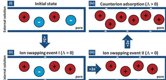
Fig. 8 (A) Fundamental electric charge compensation mechanisms: with increasing charge efficiency from (i) initial state to (ii) co-ion expulsion, (iii) ion swapping, and (iv) counterion adsorption. (B) The evolution of electric charge compensation upon increasing electrode charge, where two subsequent ion swapping events (ii) and (iii) are followed by counterion adsorption (iv).
