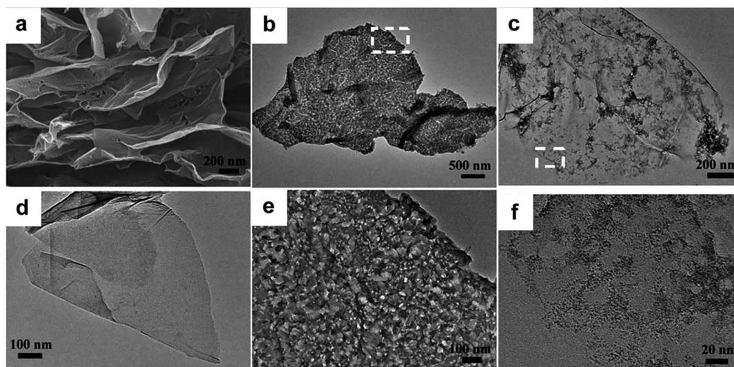
Fig. 15 (a) SEM images of rGO electrode materials. TEM image of rGO (b), rGO-PANI (c and d) and rGO-RuO<sub>2</sub> (e–f). Reproduced with permission from ref. 174. Copyright 2011 The Royal Society of Chemistry.
