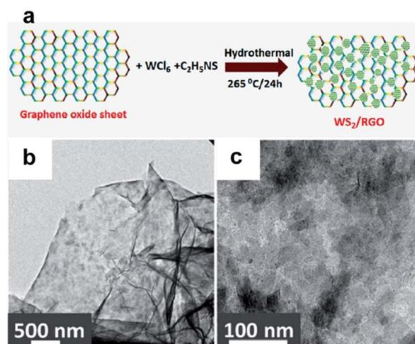
Fig. 16 (a) Hydrothermal synthesis of the WS<sub>2</sub>–rGO materials. (b and c) TEM images of the resulting WS<sub>2</sub>–rGO electrode material. Reproduced with permission from ref. 183. Copyright 2013 American Chemical Society.
