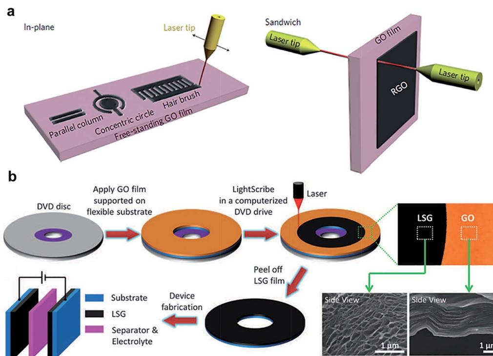
Fig. 11 (a) rGO–GO–rGO in-plane and sandwich devices obtained by laser patterning. (b) Laser-scribed graphene-based supercapacitors. Reproduced with permission from ref. 144 and 145. Copyright: 2011 Macmillan Publishers Limited and 2012 American Association for the Advancement of Science.
