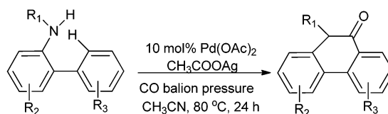
Scheme 17 Reagents and conditions: N-sulfonyl-2-aminobiaryl (50.0 mg), Pd(OAc) 2 (10 mol%), CH 3 COOAg (5 equiv.), 4 mL of anhydrous CH 3 CN, CO balloon, temp. 80 °C, time 24 h.
