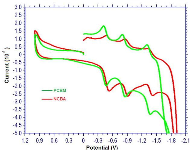
**Figure 2.** Cyclic voltammogram of NCBA (under  $N_2$ , 0.1 M  $Bu_4NPF_6$  in *o*-DCB/MeCN (4:1) solution mixture, vs Ag/AgCl; GCE as the working electrode, scan rate 0.1 V/s. internal standard  $Fc/Fc^+$   $E_{1/2}$  at 0.68 V)
