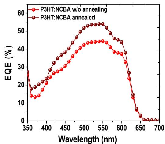
**Figure 5.** External quantum efficiency (EQE) spectra of devices based on P3HT: NCBA with and without annealing.
