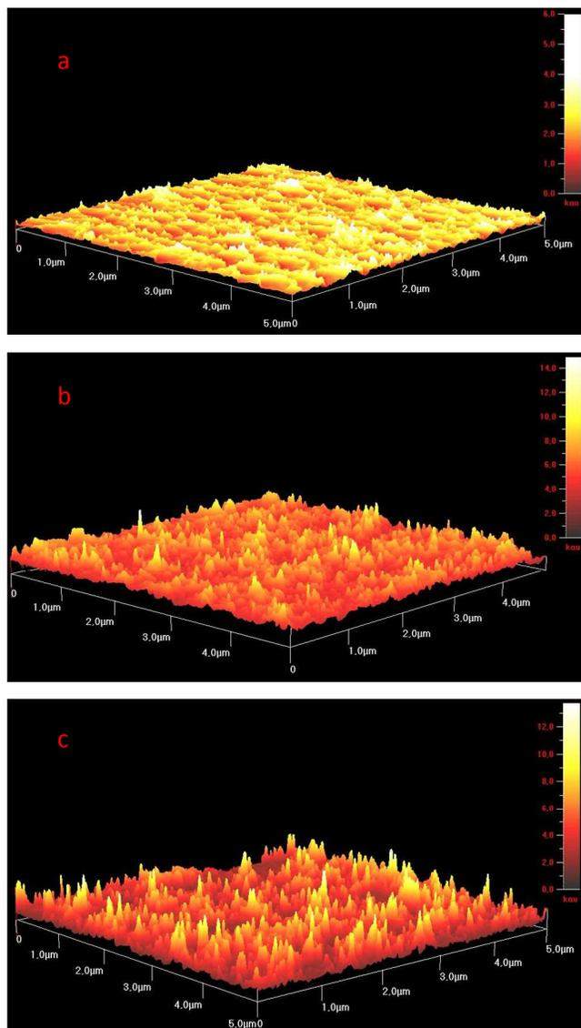
**Figure 6.** Atomic Force Microscopy (AFM) Images of NCBA:P3HT (1:1 ratio) based organic solar cells; PEDOT on ITO glass (a); NCBA on PEDOT/ITO surface before annealing (b); NCBA on PEDOT/ITO surface after annealing (c).
