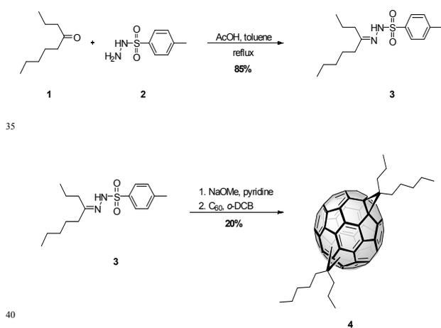
**Scheme 1.** Synthetic route to bis-4-propylpentyl [6,6] methanofullerene NCBA.
