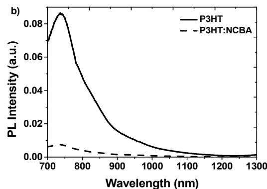
60 **Figure 1.** a) UV-vis absorption spectra of NCBA and PCBM films and b) Photoluminescence quenching of P3HT using 50% NCBA excited at 488 nm.
