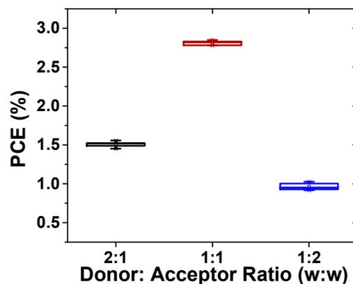
10 **Figure 4.** Average key parameters of P3HT:NCBA solar cells from 6 devices
