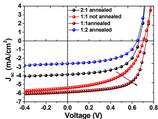
**Figure 3.**  $J$ - $V$  characteristics of P3HT: NCBA devices using different donor: acceptor ratios, under illumination at 100mW/cm<sup>2</sup>.
