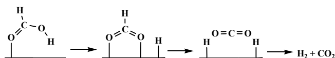
Scheme 4. General mechanism of formic acid decomposition over various surfaces through formate route.
