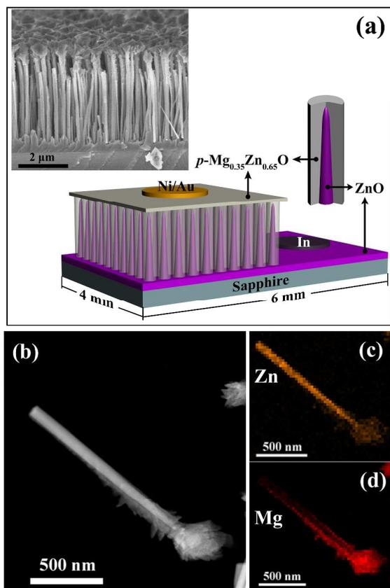
**Fig. 3** (a) Schematic diagram of the *n*-ZnO/*p*-Mg<sub>0.35</sub>Zn<sub>0.65</sub>O core-shell nanowire heterostructure, and the inset shows the side-view SEM image of the device; (b) Dark field Scanning TEM image of an individual ZnO/MgZnO core-shell nanowire heterostructure, and the EDS elemental mapping of Zn (c) and Mg (d).
