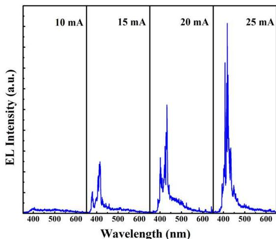
Fig. 5 Room temperature EL spectra of the heterostructure at different injection current.
