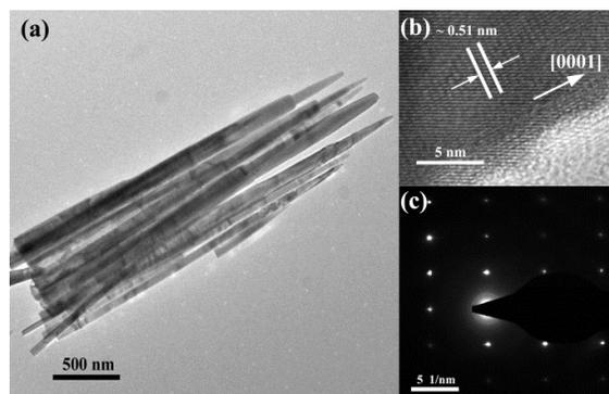
Fig. 2 TEM image of the ZnO nanowires (a); the high-resolution TEM image (b) and selected area electron diffraction pattern (c) of an individual ZnO nanowire.
