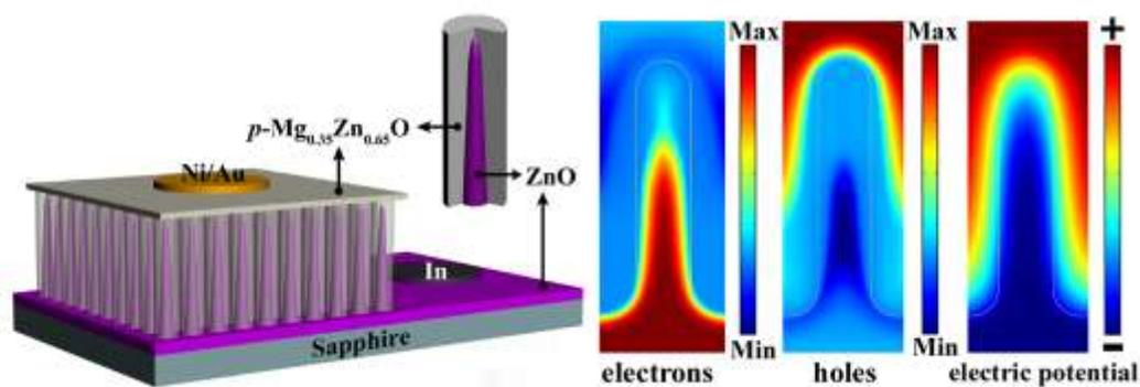
Low threshold electrically pumped random lasers were realized in  $p$ -MgZnO/ $n$ -ZnO core-shell nanowire heterostructures.
