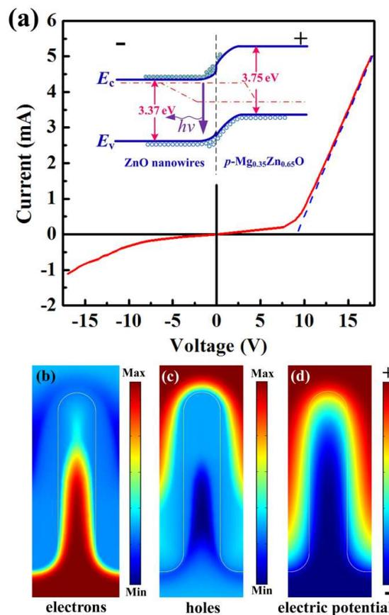
**Fig. 4** (a) *I*-*V* curve of the *p*-*n* heterostructure, and the inset shows the bandgap diagram under forward bias; (b) the electrons distribution, (c) the holes distribution, (d) the electric potential distribution in the core-shell nanowire heterostructure.
