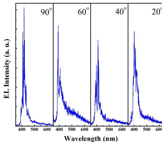
Fig. 6 Angular-dependent EL spectra of the device under the injection current of 25 mA, in which 90° means the detector is perpendicular to the surface of the sample.
