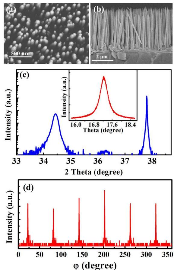
Fig. 1 Plan-view (a) and side-view (b) SEM images of the ZnO nanowires; (c) 0-20 XRD pattern of the ZnO nanowires, and the inset shows the rocking curve of the nanowires; (d) x-ray phi-scan spectrum of the nanowires.
