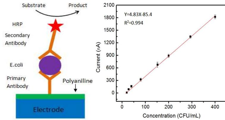
Detection of *E. coli* O157:H7 in beef juice with a detection limit of 19 CFU/mL. An assay time of 67 min was resulted due to the absence of sample pre-enrichment.
