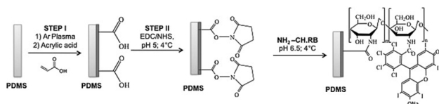
Fig. 4 Schematic illustration of the different steps for PDMS surface modification with CH. RB. Reprinted from ref. 129 Copyright (2013), with permission from Elsevier.
