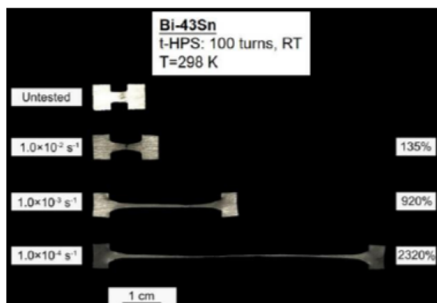
Fig. 8 An example of superplasticity in a Bi-43% Sn alloy after processing by t-HPS. 87
