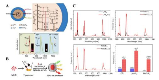
Fig. 2 (A) Energy transfer mechanism in the NaErF<sub>4</sub>:2%Ho@NaYF<sub>4</sub> core/shell UCNPs and the upconversion emission spectrum of the obtained NIR-II UCNPs.<sup>16</sup> (B) Schematic illustration of the synthesis of the series of core—shell upconversion nanoparticles.<sup>17</sup> (C) UC emission spectra of core—shell nanoparticles, and the integration of their emission peaks excited at 1532 nm.<sup>18</sup>
