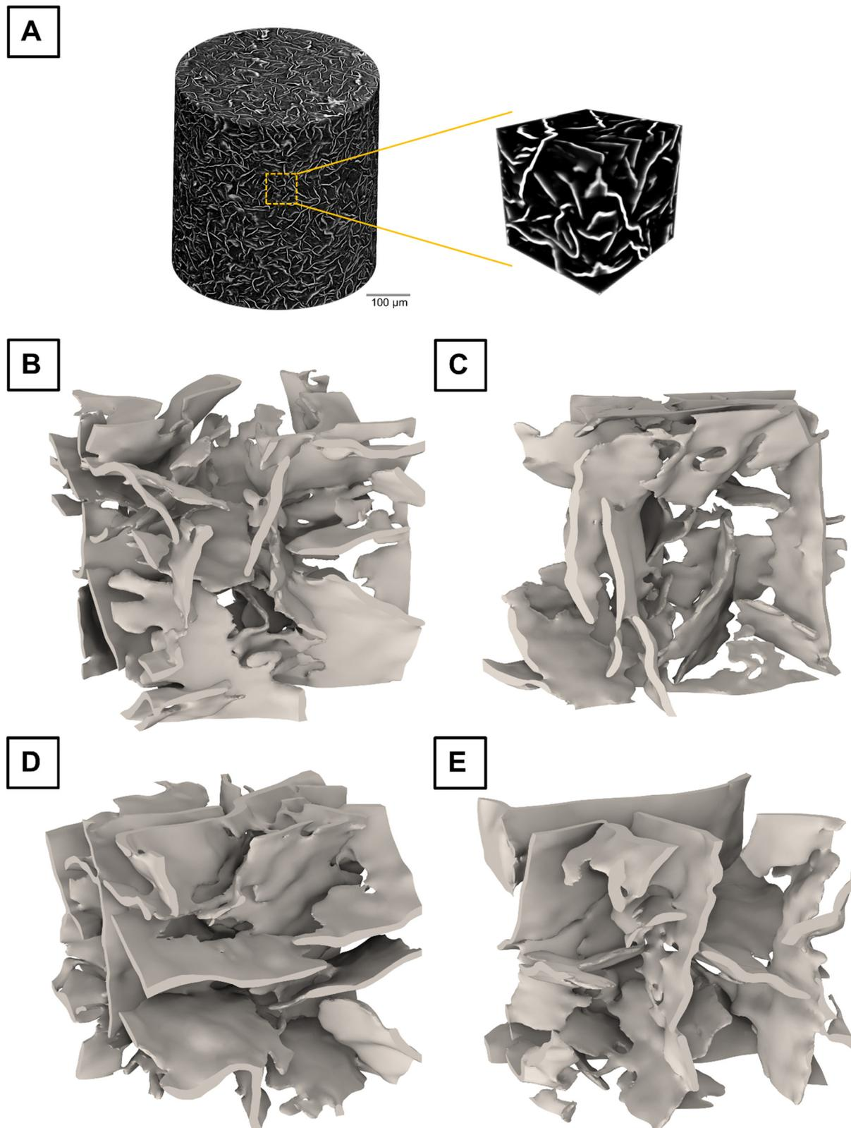
**Fig. 1** (A) Full 3D tomographic reconstruction of a monoglyceride-based oleogel obtained by phase-contrast X-ray tomography. The dark colors are regions of liquid oil, whereas the bright colors are solid monoglycerides. Microscopic representative volume elements (RVEs) are sampled from the full reconstruction. (B)–(E) Examples of RVE revealing the microscopic structure of the monoglyceride crystal network. The edge size of the RVE cube is 60 μm.
