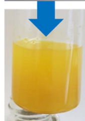
Fig. 5 An inverse vulcanised polymer that has undergone an auto-acceleration during its synthesis. Bubbles can be seen throughout its structure as auto-accelerations in inverse vulcanisation are associated with increased hydrogen sulfide generation. Note the inhomogeneity in the polymer.
