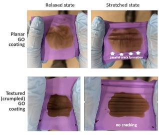
Fig. 10 Demonstration that compressive pre-texturing of graphene oxide films renders them stretchable, with no cracks observed over multiple stretch and relax cycles. Films (0.5  $\mu m$  thick) were formed by solution casting of pure graphene oxide (no polymer additive) on nitrile glove cutouts. Still images extracted from video original (see Videos S1 and S2†).
