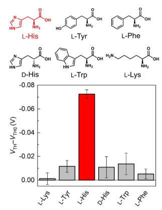
Fig. 4 Selectivity test results of the MIP-OFET for amino acids (1.0 mM) in a phosphate buffer solution (100 mM) at pH 6.0 at 25 °C. The terms  $V_{\rm THO}$ and  $V_{TH}$  mean threshold voltages before and after adding targets (n = 3).
