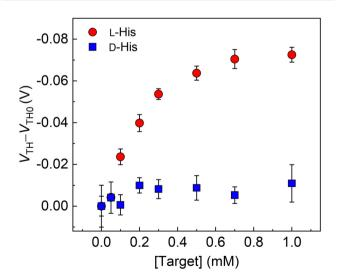
Fig. 3 Responses of the MIP-OFET to L-(red circles) and D-His (blue squares) in a phosphate buffer solution (100 mM) at pH 6.0 at 25  $^{\circ}$ C. The terms  $V_{\mathrm{TH0}}$  and  $V_{\mathrm{TH}}$  mean threshold voltages before and after adding targets (n = 3). The titration isotherms were obtained by collecting  $V_{TH}$ s at  $V_{\rm GS} = -2 \text{ V}.$
