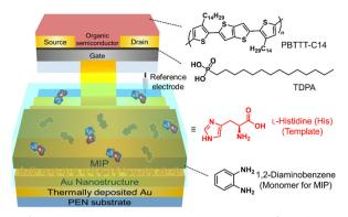
Fig. 1 Schematic illustration of an extended-gate-type OFET functionalized with MIP for chiral recognition and % ee determination of L-His and chemical structures of the sensor components. 1,2-Diaminobenzene was used as the functional monomer for MIP fabrication.
