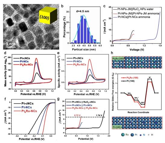
Fig. 8 (a) TEM image and (b) size distribution of Pt-NCs. (c) LSV curves of Pt-NPs-JM and comparison sample in ammonia electrolyzer. Represented the Amoretical Copyright 2020, Elsevier. (d) Mass and (e) specific activities of the Amoretical Copyright 2020, Elsevier. (d) Mass and (e) specific activities of the Amoretical Copyright 2020, Elsevier. (d) Mass and (e) specific activities of the Amoretical Copyright 2021, Represented the Copyright 2021, Royal Society of Chemistry.
