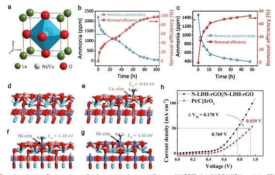
Fig. 10 (a) Perovskite structure. Concentration profile of ammonia and removal efficiency of LNCO55-Ar in (b) 0.5 M KOH containing 2210 ppm NH<sub>4</sub>Cl and (c) real wastewater with 0.5 M KOH. (d) The calculation model of LaNi $_{0.5}$ Cu $_{0.5}$ O $_{3-\delta}$ . (e)–(g) Configuration diagram of ammonia molecule adsorbed on different sites. 85 Copyright 2021, Wiley-VCH. (h) LSV curves of N-NiZnCu LDH/rGO and commercial Pt/C||IrO2. 84 Copyright 2020, Elsevier.
