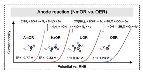
Fig. 2 Comparison of various electrocatalytic oxidation reactions of nitrogenous substances with the OER
