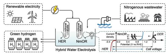
Fig. 1 Schematic of H<sub>2</sub> generation from renewable energy-powered HWE systems in nitrogenous wastewater
